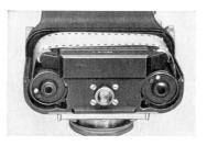
c) Inserting the cassette and closing the camera
