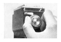
3. Wind the shutter by turning the knob 2 in the direction of the arrow as far as the stop.
