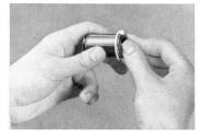
2. Press the nickelled cap and turn until the two openings of the sleeves are superimposed.
