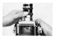
camera lens snaps into place and rotates with it. With lenses of a longer focal length than 2", the focusing should be done by turning the focusing arrangement on the taking lens, as the gear ratio of the focusing lever is too high for such focal lengths.
