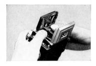
When closing the hood, fold back first the two side flaps 10, then the Albada finder lens 11 and
