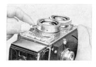
Focusing on the ground glass screen is done by movement of the lever 13 on the lens 14, which is coupled with the picture-taking lens 15.
