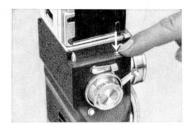
Pressure on the button 22 operates the delayed action release, which can be used within the range of the shutter speeds. When the shutter is set to B, the length of exposure in conjunction with the delayed action release will be about 1 second. Even with the clock-work set, the shutter can be released by pressing down the lever 7 and then wound again.
