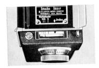
6. When the illumination is very poor, it will be impossible to bring the pointer as far as the index mark, even when the lever 29 is moved to its extreme position. It is then necessary to read off the exposure time indicated and multiply it by a factor resulting from the position of the pointer on the scale between zero point and index mark. The lines seen in the window have their corresponding lines in the table fixed to the flap of the hood and indicated immediately above.
