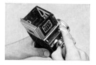
A pressure on the button 9 causes the hood to spring into position.
