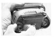
4. Detach the gummed strip of the film (carefully, so that the spool does not unroll). Place the spool on the take-up studs of the left spool chamber 3.
