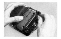
Wind paper on to the empty spool until the line at the arrow lies on the transport sprocket 5 when placing the spool in the right spool chamber 4.
