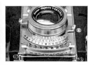
5. The appropriate exposure time on the scale 30 can be read off for every diaphragm, or conversely, the correct diaphragm can be read off for the desired time of exposure. The black numbers on the scale 30 denote fractions of a second, e. g.  $25 = \frac{1}{25}$ th second,  $2 = \frac{1}{2}$  second. The red numbers indicate full seconds. Allowance can be made for intermediate values by a corresponding adjustment of the diaphragm.
